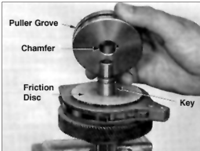
Figure 5-7. View Showing Load Brake Flange Removed
