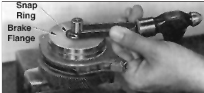
Figure 5-6. Remove Snap Ring From Load Brake Shaft
